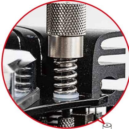
Do not over-tighten the thumb screws. The springs should be slightly compressed, with visible gaps in the spring coils. Over-tightening may result in poor contact between the water block and CPU.
