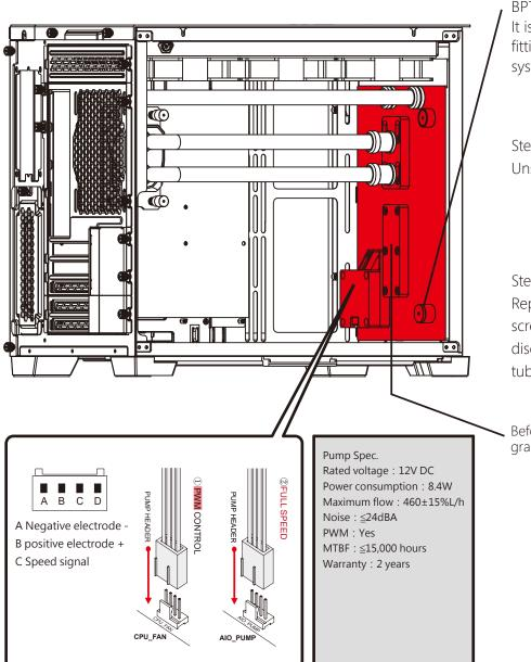
BPTA-EFW It is recommended to install the water-exhaust fitting at the lowest point of the water cooling system.
