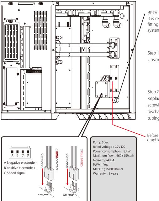
**BPTA-EFW** It is recommended to install the water-exhaust fitting at the lowest point of the water cooling system.
