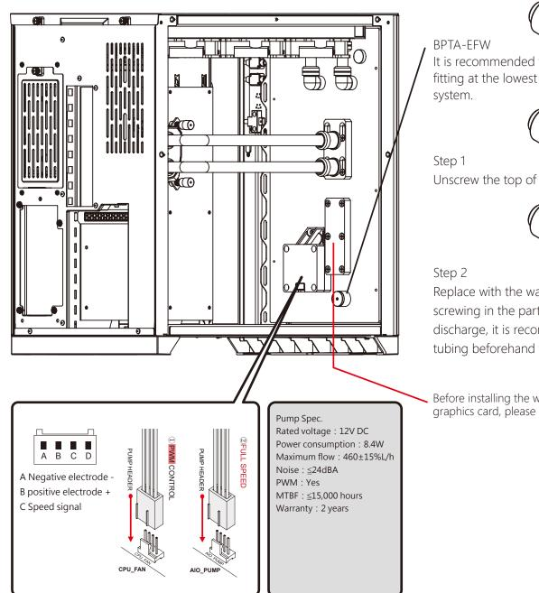
It is recommended to install the water-exhaust fitting at the lowest point of the water cooling system.
