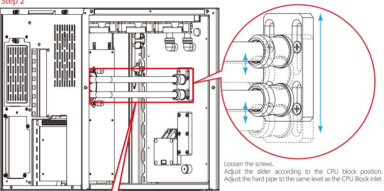
When installing the hard pipe from the CPU block to the water distribution reservoir, You can move the hard pipe left and right to get the proper installation length.
